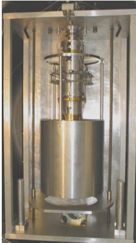
Figure 5.1 The GGG apparatus mounted in a metal frame fixed inside a vacuum chamber (not shown) of 1m diameter.
