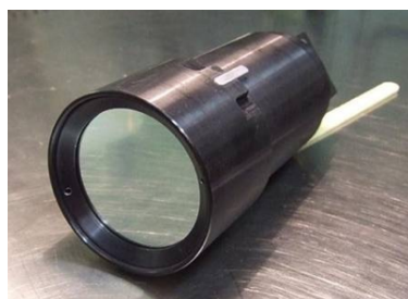
Figure 15: Fully integrated spin rate sensor breadboard (realized within 2009 ASI study)
