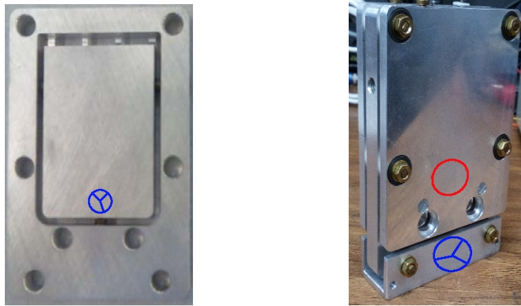
Figure 11: Test mass selected. On the left it is shown stand-alone. Four lamellae suspending the plate from the top are visible. In the picture to the right the same mass is integrated with the base structure –by means of 2 screws at the bottom– and located in between two capacitance plates which serve as pick-up plates, forming a capacitance bridge which allows to detect the displacements of the test mass from its equilibrium position in between them. The gaps between the test mass and each plate are kept at 500\ \mu\text{m} by teflon washers. In blue are shown the locations where two corner cube reflectors shall be installed, one to serve as target point on the test mass and one on the base structure (right) to serve as reference point relative to which the displacements of the test mass will be detected by our laser interferometer. The red circle depicts the location on the capacitance plate where a hole shall be made for the laser to reach the corner cube reflector on the test mass. Thus, it will be possible to read the displacements of the test mass, at the same time, by the capacitors and by the laser interferometer.
