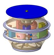
The GG satellite. 400 kg total mass, 1.4 m width, 1.2 m height to be flown in a standard near circular, low altitude ( $\simeq 600$  km) sun-synchronous orbit for a 9-month mission duration.
