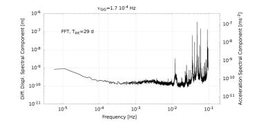
At  $\nu_{\rm GG} \simeq 1.7 \cdot 10^{-4}$  Hz the measured relative displacement SD is  $\simeq 1.8 \cdot 10^{-7} {\rm m}/\sqrt{{\rm Hz}}$  and the measured relative acceleration SD is  $\simeq 6 \cdot 10^{-8} {\rm ms}^{-2}/\sqrt{{\rm Hz}}$
