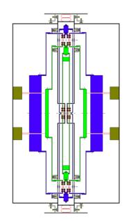
Section of GG balance along symmetry/rotation axis. Inner and outer test cylinder (green and blue) are suspended at their centers of mass from the PGB (an intermediate suspension stage sketched with a rectangular section) which encloses the sensor, screens it from various disturbances and mounts instrumentation (here the read-out laser gauge is shown)
