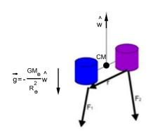
$\vec{F_1}$  and  $\vec{F_2}$  are the forces acting on each mass. Their vectorial sum applied to the center of mass CM is balanced, on the ground, by the suspension fiber directed along  $\hat{w}$  (to the center of mass of the Earth). Only the component of the total torque along  $\hat{w}$  does twist the wire. It is found to be:
