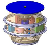
Note the cylindrical symmetry. Attitude stabilization is by rotation around symmetry axis
