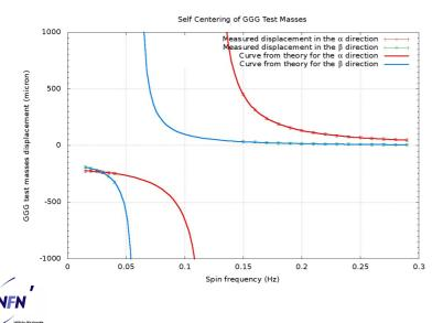
Experimental data from the GGG accelerometer agree with the theoretical curves in both directions  $\alpha$ ,  $\beta$  of the rotating plane:
