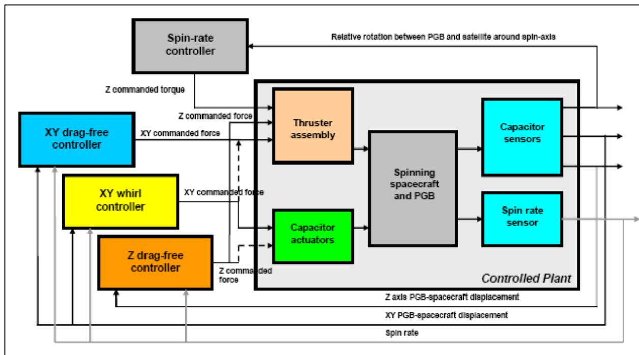
**All controllers designed according to state-space approach based on state observer and gain feedback functions**
