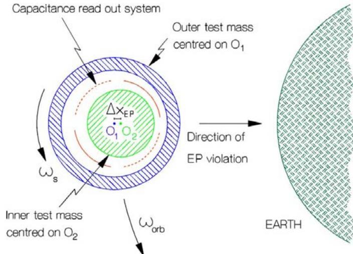
**Objective: 0.5 pico-m displacement between 2 rotors in supercritical rotation**
