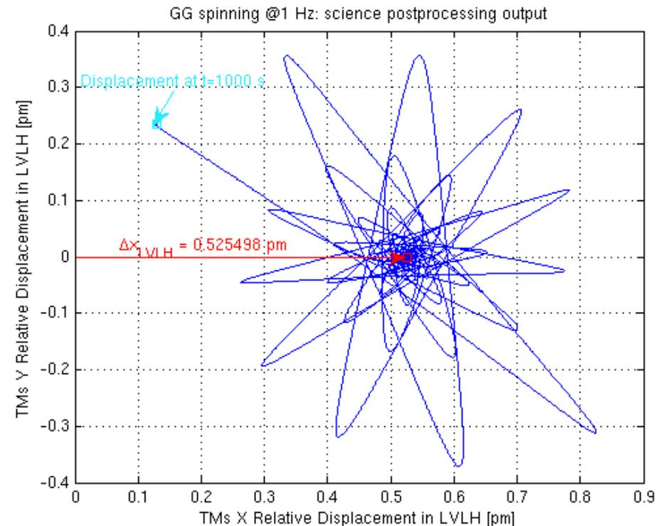
Polar plot of the differential displacement in the local vertical – local horizontal reference (LVLH) frame. After a transient, the TMs relative displacement has nearly null mean value along  $Y_{LVLH}$  and 0.525 µm mean value along  $X_{LVLH}$
