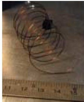
Figure 9.B.3: One suspension spring made of 1 steel wire and 3 Cu wires.
