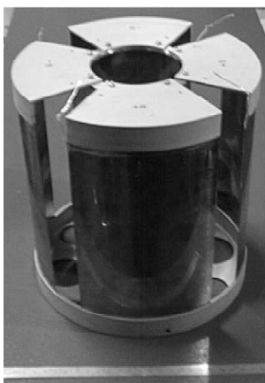
Fig. 5. The four capacitance plates (with their insulating frames) forming the two capacitance bridges of the read-out. They are mounted halfway in between the concentric test cylinders to read their relative displacements (see section in Fig. 2).
