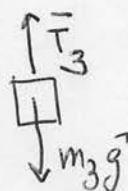
$$\left. \begin{array}{l} m_1 \vec{a}_1 = \vec{N}_1 + m_1 \vec{g} + \vec{T}_{12} + \vec{T}_{13} \\ m_2 \vec{a}_2 = \vec{N}_2 + m_2 \vec{g} + \vec{T}_2 \\ m_3 \vec{a}_3 = \vec{N}_3 + m_3 \vec{g} + \vec{T}_3 \end{array} \right\}$$
