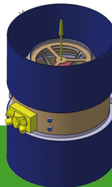
Fig. 3 The GG cylindrical spacecraft (1.45 m central diameter) showing the solar panels (blue), the main body (light brown, see fig. 4) with one of the two antennas along the symmetry axis.
