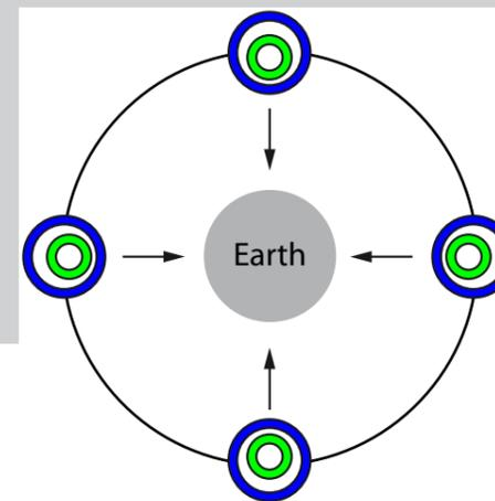
Fig. 2 The EP violation signal in GG. Section in the plane perpendicular to the spin/symmetry axis of the GG outer (dark blue) and inner (green) test cylinders (of different composition and weakly coupled in the plane) as they orbit around the Earth inside a co-rotating, passively stabilized spacecraft (not shown). The centers of mass
