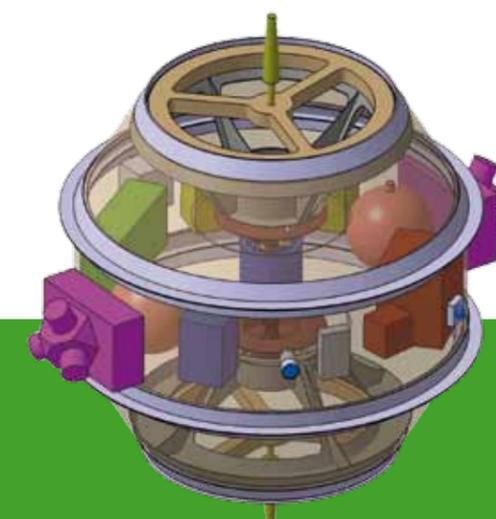
Fig. 4 Transparent view of the spacecraft body (shown in fig. 3 with the solar panels). At its center the outer test cylinder of the GG accelerometer is visible in blue.
