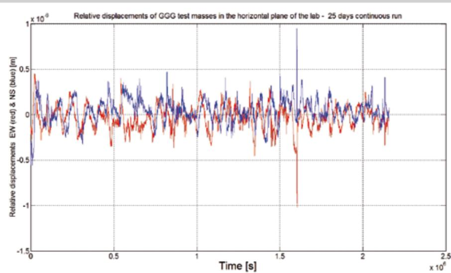
Fig. 9 Relative displacements of the GGG test cylinders in the East-West (EW) and North-South (NS) directions of the horizontal plane of the lab as a function of time during a 25 days continuous run. A single isolated jump occurs; other than that, the amplitude of the displacements is of  $2 \times 10^{-7}$  to  $4 \times 10^{-7}$  m (the diurnal pattern is apparent).
