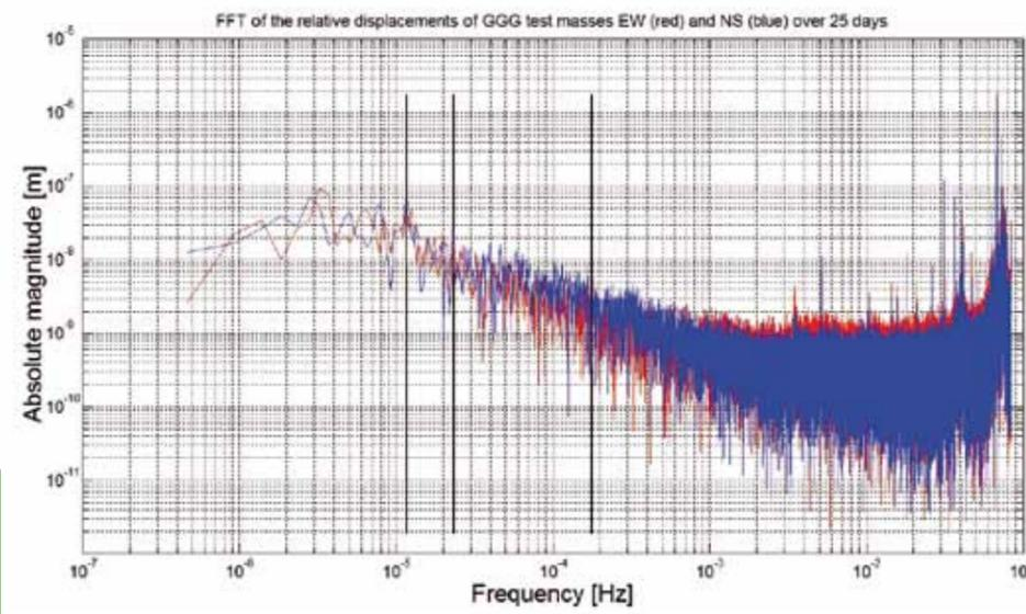
Fig. 10 Fast Fourier Transform of the relative displacements of the GGG test masses whose time variation in the EW and NS directions of the horizontal plane was shown in fig. 9. The 3 vertical black lines indicate (from left to right) the frequencies corresponding to 24 h, 12 h and
