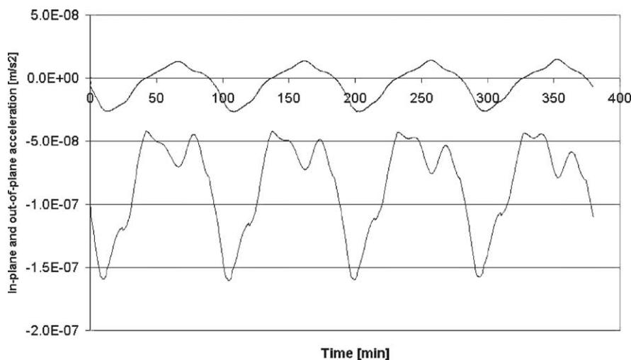
Fig. 4. Perturbing accelerations in the measurement plane and perpendicular to it, when the spin axis is  $10^\circ$  away from the orbit normal (summer solstice 2005). The magnitude of the out-of-plane acceleration (top) is less than  $1/6$  of the in-plane component (bottom).
