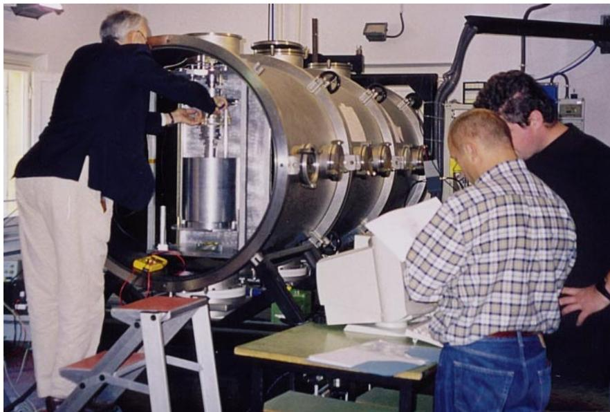
Figure 3.4 The rotor designed in Fig. 3.1 being mounted by Dr. D. Bramanti inside the vacuum chamber in the laboratory of LABEN in Florence. The electronics was in part realized by QSA Srl, Arezzo
