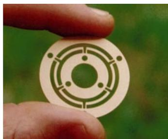
Figure 2.3 One of the two flat gimbals to be used for coupling the GG test bodies (as shown in Fig. 2.1). The outer ring is clamped to the PGB tube and the inner one to the coupling arm (in Fig. 2.1 the PGB tube is shown in dark green and the coupling arm in light blue). There are 6 wire sectors in between the clamping rings; 3 of them (in
