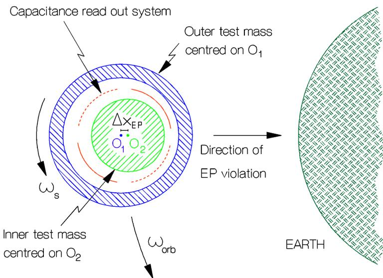
EP violation signal on the GG test bodies modulated at the spin frequency of the system ( 2 Hz )
