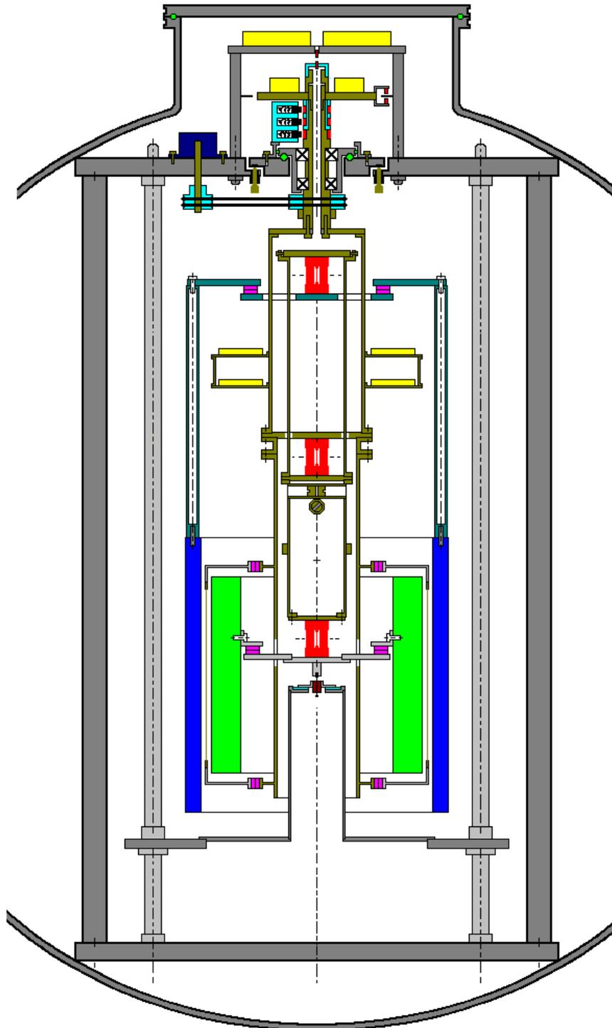
Sketch of GGG apparatus mounted inside vacuum chamber (1 m diameter)
