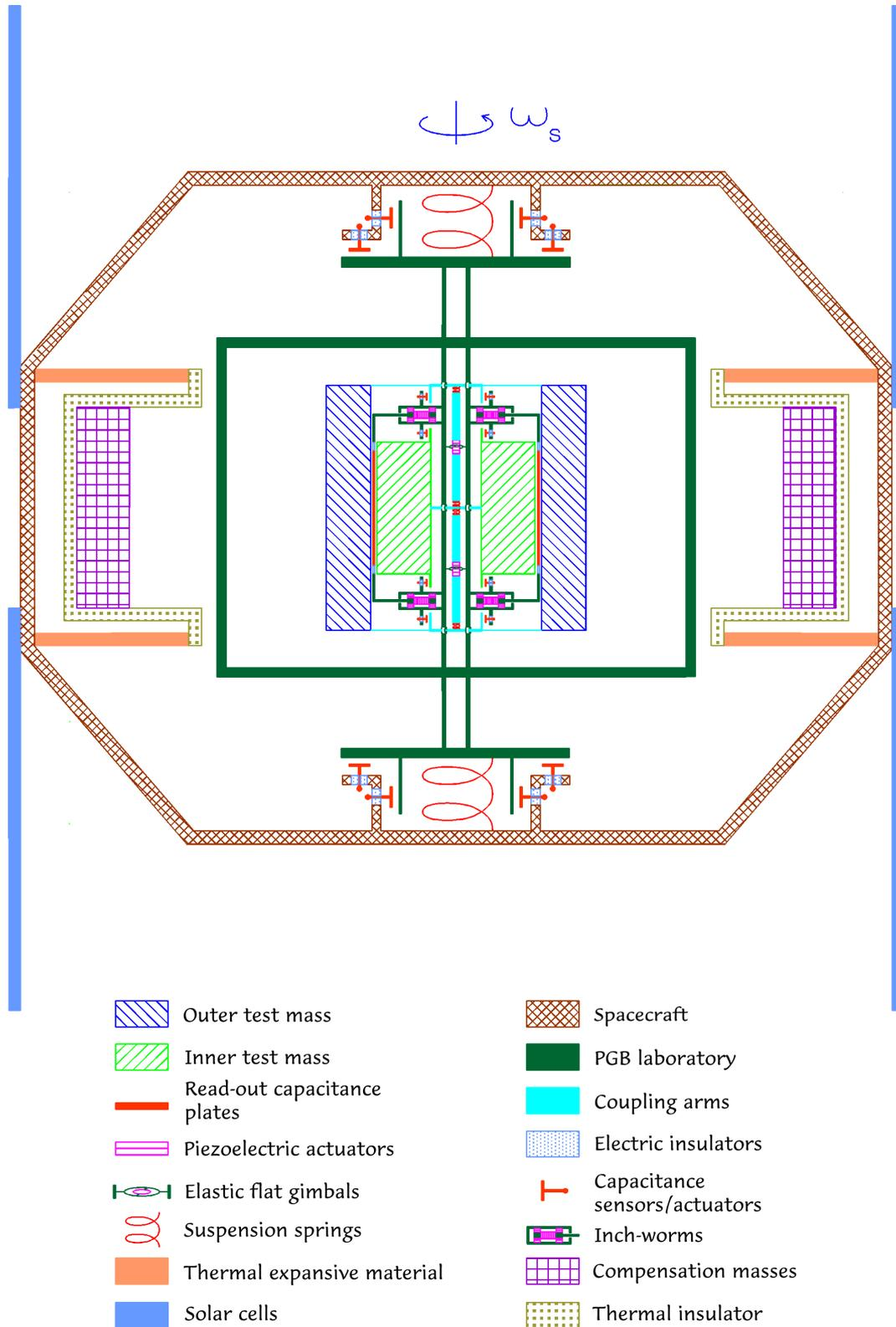
Section of the GG s/c through its spin axis
