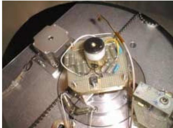
Led used for optical transfer of signals from the rotating apparatus to the non rotating frame (then transferred outside the vacuum chamber and acquired by the computer)
