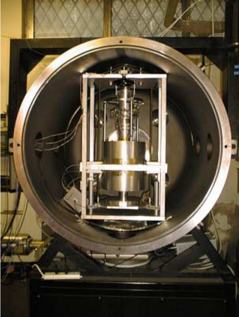
The GGG apparatus inside the vacuum chamber (in the basement of the laboratory)
