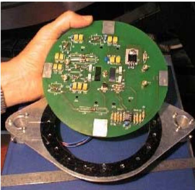
Electronics for optical transfer (20 signals per turn, with information on phase)
