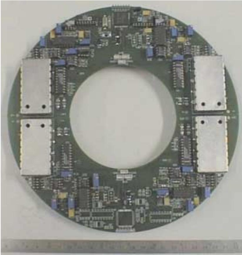
The electronics of the read-out bridges (doubled for redundancy and symmetry)
