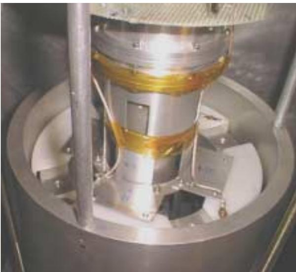
The capacitance plates (forming the two bridges of the read-out system) mounted in between the test cylinders (system operational at 6 Hz rotation rate)
