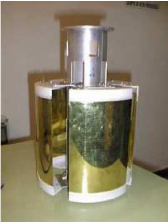
The GGG capacitance plates for measurement of relative displacements. On bench:  $5 \cdot 10^{-12}$  m in 1 sec integration time; with full GGG system operational at 6 Hz rotation:  $10^{-9}$  m s<sup>-2</sup>/√Hz
