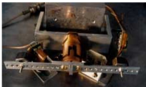
Figure 12. One of the GGG laminar suspensions clamped and mounted for Q measurement in horizontal oscillations at a few Hz. The largest value obtained was 2,000; it improved at lower amplitudes but the measurements then became limited by seismic noise. A collaboration is underway with the University of Rochester (Department of Mechanical Engineering), in order to identify materials with higher Q which could be used to manufacture the suspensions of GGG and GG.
