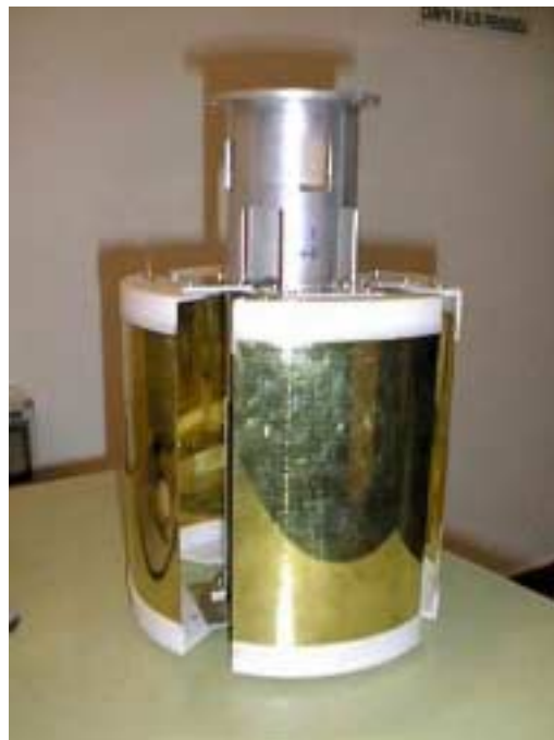
Figure 13. View from the top of the GGG test cylinders (10 kg each) one inside the other. The four capacitance plates of the read-out located in between them can be recognized (see next Figure). The electronics is visible; the coupling arm and the 3 laminar suspensions are not visible.
