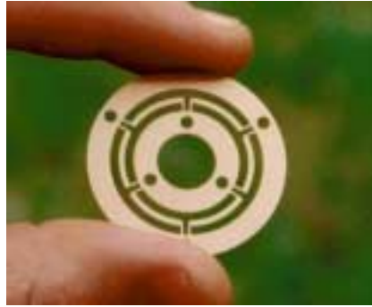
Figure 6. One of the 2 flat gimbals to be used for coupling the GG test bodies (see Figure 4). The outer ring is clamped to the PGB tube and the inner one to the coupling arm (in Figure 4 the PGB tube is shown in dark green and the coupling arm in light blue). There are 6 wire sectors in between the clamping rings; 3 of them (in alternation) carry electric signals and are insulated at the clamping (on the outer and inner clamping rings); no electric insulation is needed on the thin wires themselves where deformations occur. The manufacturer of the gimbals is the same as for the helical spring; the same heat treatment and cleaning procedure have been applied.
