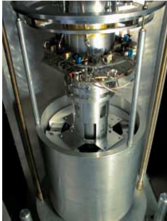
Figure 13. View from the top of the GGG test cylinders (10 kg each) one inside the other. The four capacitance plates of the read-out located in between them can be recognized (see next Figure). The electronics is visible; the coupling arm and the 3 laminar suspensions are not visible.
