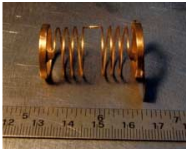
Figure 5. One of the 4 helical springs to be used for suspending the GG test bodies; two such springs are needed for each test body (see Figure 4). This spring has been manufactured in CuBe by DG Technology Service, Parma (Italy) according to our design. They have manufactured the spring by electroerosion in 3D from a single piece of CuBe with special equipment, and then have applied Brush-Wellman heat treatment and ultrasound cleaning. The elastic properties are close to the desired ones. Each spring is clamped by the thick rings at its ends. Half turns of this spring are clockwise and the other half counter-clockwise; this is for de-coupling torsional from longitudinal (axial) oscillations. No electric signal is required to pass through these helical springs.
