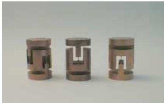
Figure 10. The three laminar suspensions of the GGG apparatus. They have been manufactured in CuBe by electroerosion in 3D following the same procedure as for the GG helical springs (see Figure 5).
