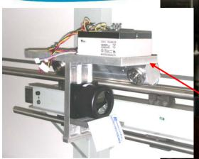
Laser interferometer breadboard under the functional test over a long distance (~90 m) with a moving target. The effectiveness of the measurement beam chopping scheme was successfully verified in this test.
