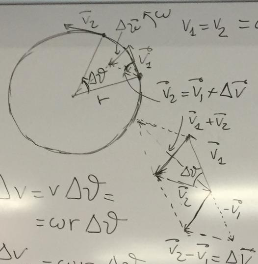
$\Delta v = v \Delta \vartheta = \omega r \Delta \vartheta$
