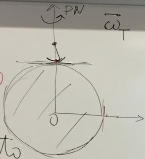
$$\frac{\vec{F}_{cor}}{m} = \vec{a}_{cor} = -2\vec{\omega}_T \times \vec{v}_{ROT}$$
