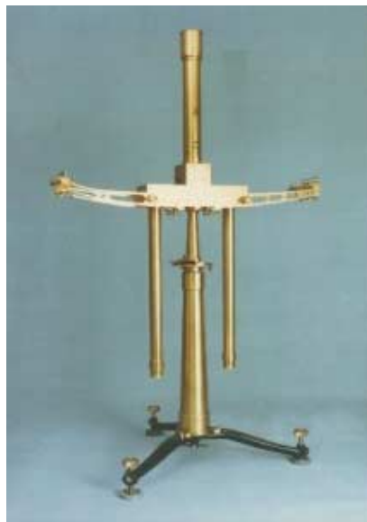
Fig. 1. – The torsion balance used by Loránd Eötvös to test the proportionality between inertial and gravitational mass. The experiments were carried out starting in 1888, and then in the period between 1905 and 1908. (Picture downloaded from the Eötvös virtual museum available on the World Wide Web).
