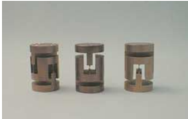
Fig. 12. – The 3 laminar suspensions of the GGG apparatus. They have been manufactured in CuBe by electroerosion in 3-D to ensure good mechanical quality.
