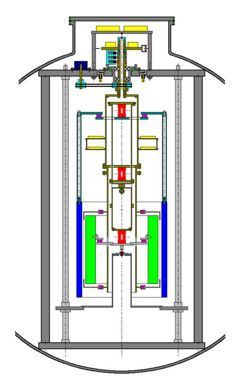
Sketch of GGG apparatus mounted inside vacuum chamber (1 m diameter)
