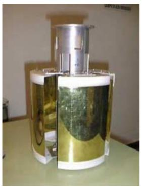
The GGG capacitance plates for measurement of relative displacements. On bench:  $5 \cdot 10^{-12}$ m in 1 sec integration time; with full GGG system operational at 6 Hz rotation:  $10^{-9}$  m s<sup>-2</sup>/ $\sqrt{Hz}$
