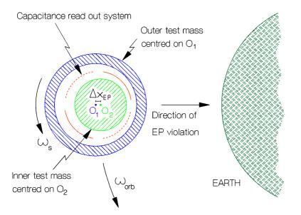
EP violation signal on the GG test bodies modulated at the spin frequency of the system (2 Hz)
