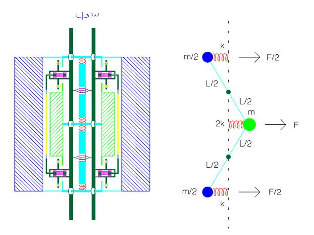
Section of test cylinders showing that they are coupled like in an ordinary balance (with vertical beam) so that common mode effects can be rejected by adjusting the length of the arms by means of PZT actuators
