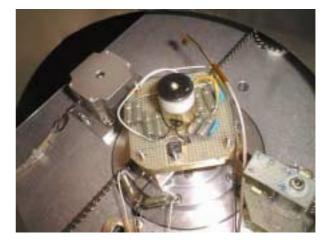
Led used for optical transfer of signals from the rotating appartus to the non rotating frame (then transferred outside teh vacuum chamber and acquired by the computer)
