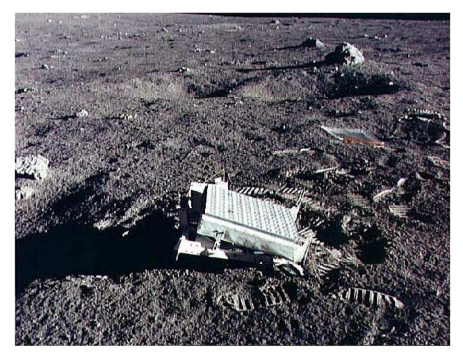
The retroreflector array of Apollo 14 on the lunar surface
