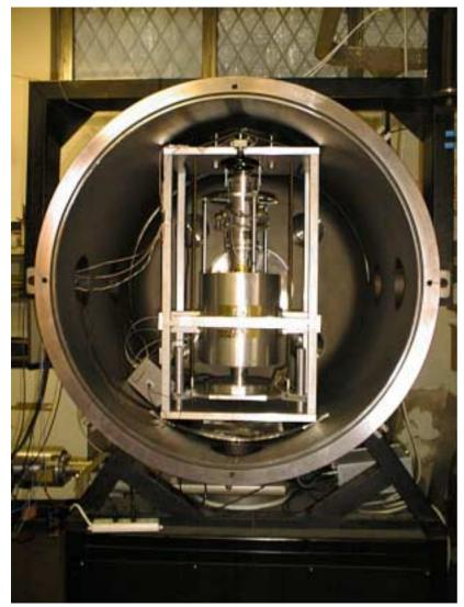
The GGG apparatus inside the vacuum chamber (in the basement of the laboratory)
