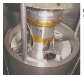
The capacitance plates (forming the two bridges of the read-out system) mounted in between the test cylindres (system operational at 6 Hz rotation rate)
