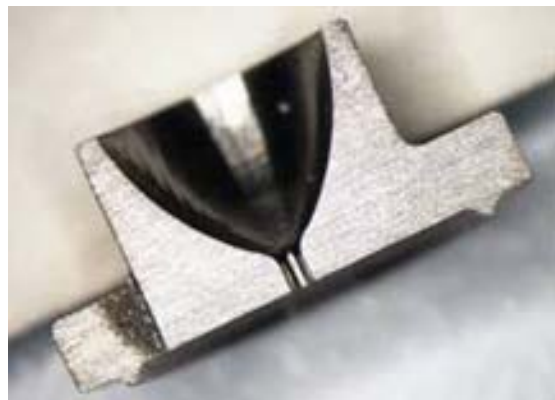
Low Pressure Regulation Valve with Nozzle (cutaway) close up
