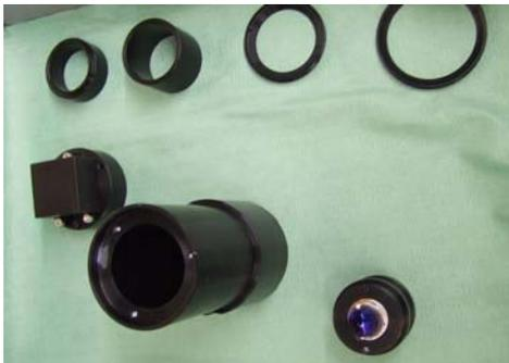
From left to right: (top) spacers and retaining rings; (bottom) detector box, sensor body, internal optics barrel
