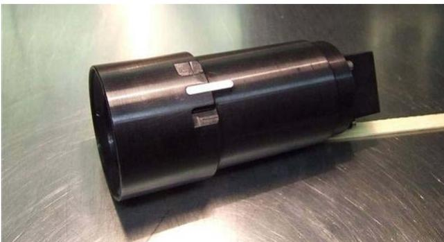
Fully integrated spin rate sensor
