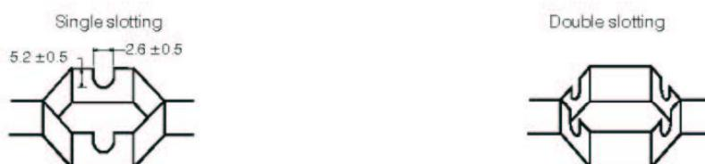
Maximum slice thickness for slotted honeycomb 51mm for all cell sizes
