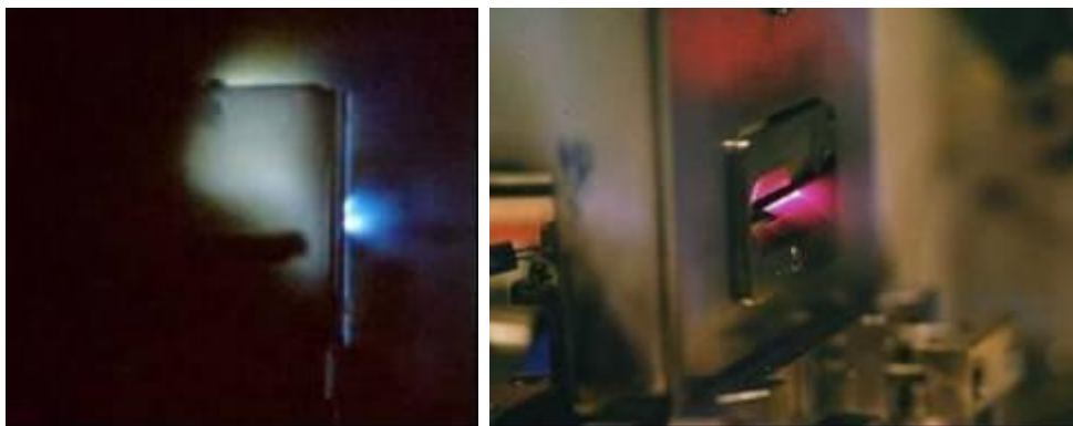
Figure 2.4: Alta's FEEP thrusters firing with Cs (left) and Rb (right) propellants.
