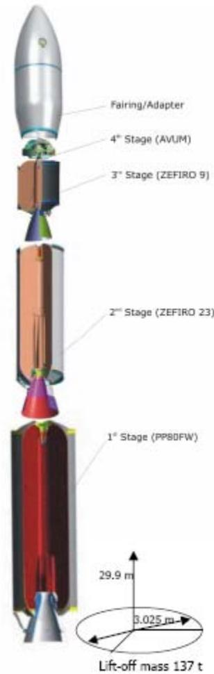
**Figure 5.2-1: VEGA launch vehicle schematic architecture**
