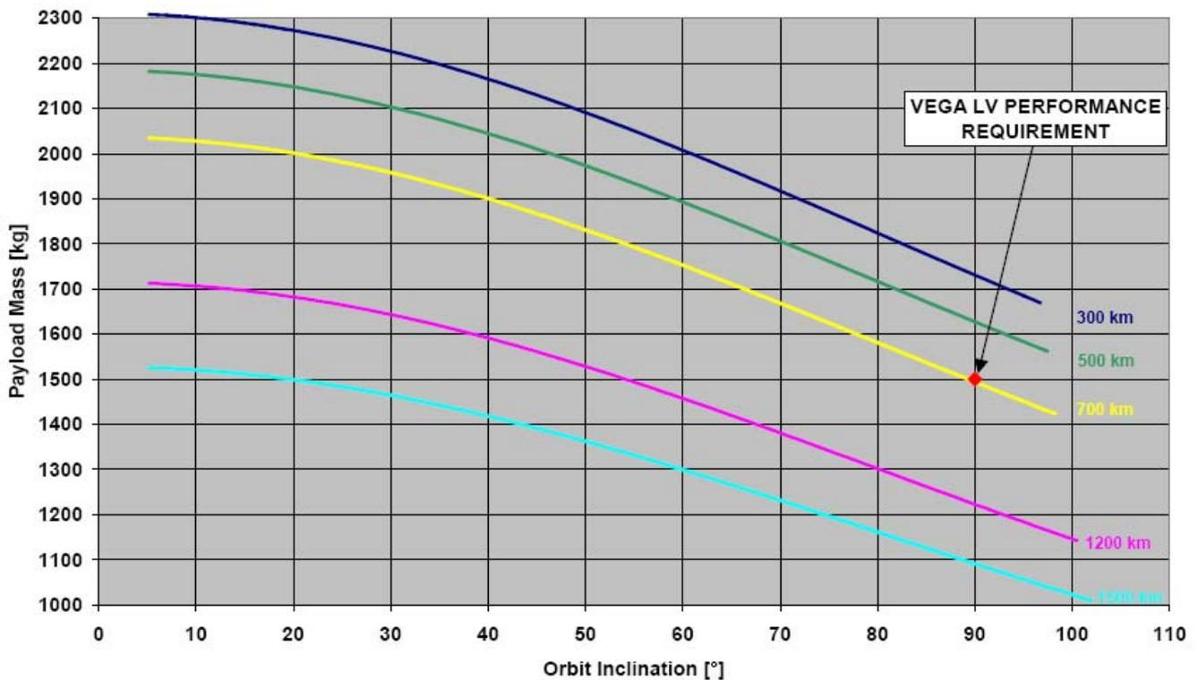
Figure 5.2-2: VEGA performances for circular orbits (source: [RD 31])
