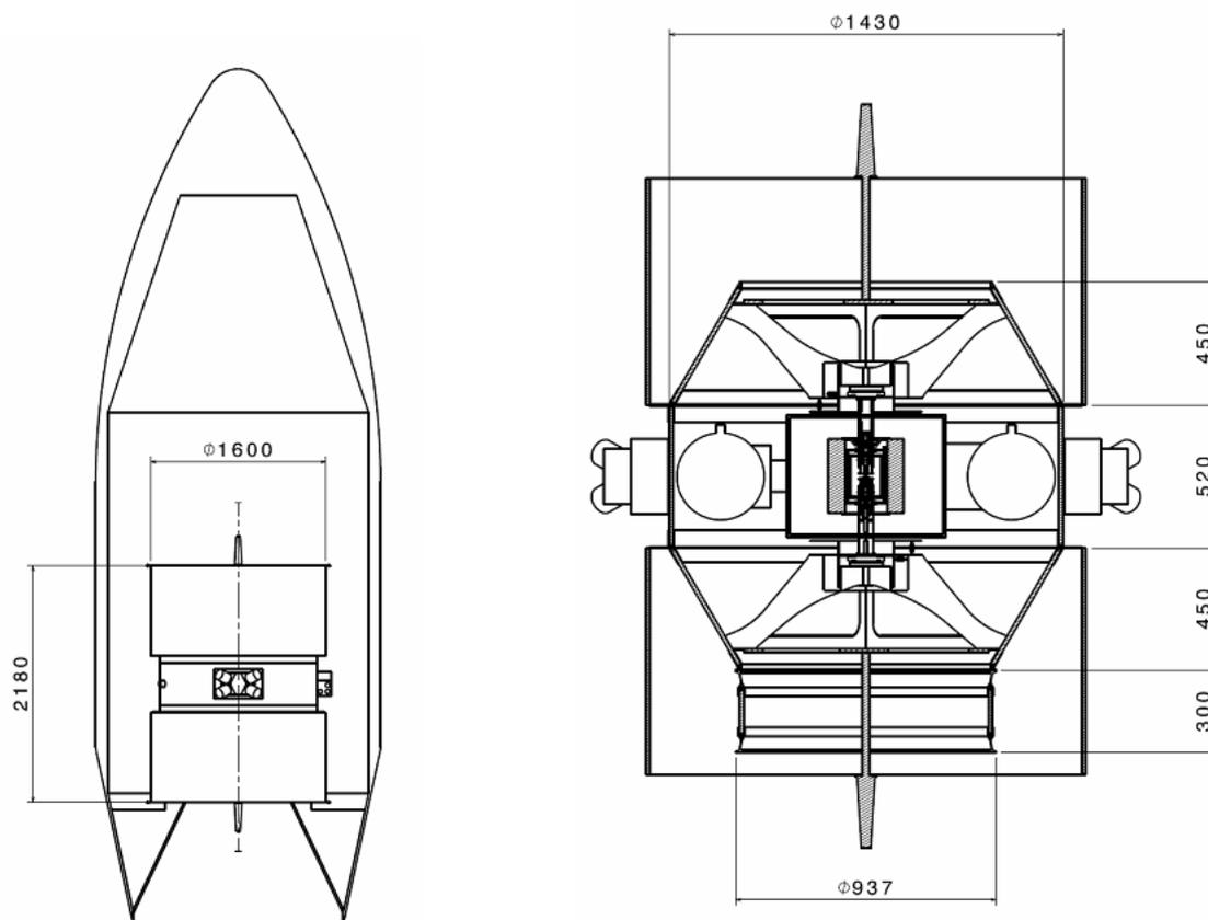
**Figure 4.1-1: GG spacecraft configuration and main dimensions**
