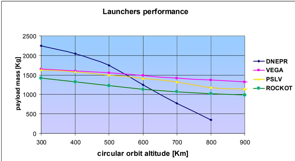
Figure 4.3-3: Payload mass capability for DNEPR, VEGA, PSLV and Eurockot
