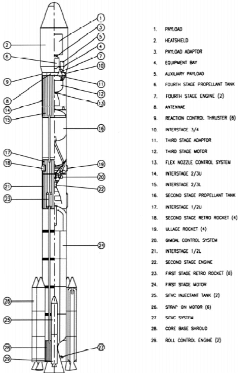
Figure 5.3-1: PSLV launch vehicle schematic architecture (source: [RD 32])
