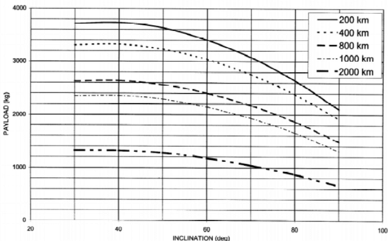
Figure 5.3-2: PSLV performances for circular orbits (source: [RD 32])
