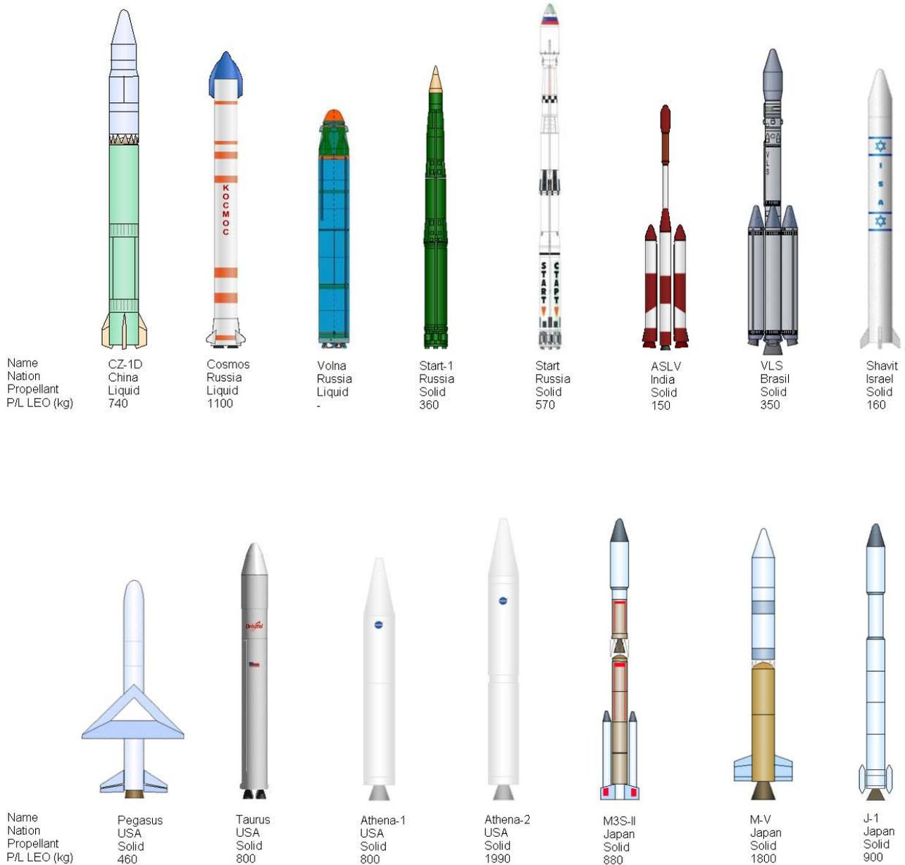
Figure 4.3-1: Small launchers review (pictures not in scale)
