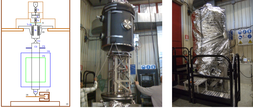
Figure 3: In order to isolate the GGG rotating accelerometer from low frequency terrain and ball bearings noise (tilts as well as horizontal accelerations) the current design ( left ) exploits the attenuation provided at low frequencies by the 2D flexible joint (labeled 11r) isolating the upper part of the shaft (9r) –which is subject to ground tilts and ball bearings (8) noise– from the lower part (12r) which holds the GGG balance. Thus, the isolated part of the shaft (12r) is driven by its weight closer to the direction of local gravity (which defined the vertical direction) more than its tilted top part. The central picture shows the experimental apparatus while opening the vacuum chamber. The picture to the right shows the vacuum chamber closed with thermal insulation in place.
