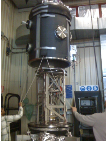
Figure 1: Left : the GGG apparatus (at INFN lab in San Piero-Pisa, built with ASI and INFN funding). The proof masses are concentric cylinders (10 kg each) with the symmetry axis in the vertical direction, weakly coupled in the horizontal plane by high quality CuBe joints in 2D. Together they form a very peculiar beam balance in which the beam is vertical –hence the balance is sensitive to differential forces in the horizontal plane– and the masses are concentric. The relative displacements of the cylinders in the horizontal plane are read by 2 orthogonal capacitance bridges whose plates are located halfway in between them. The balance rotates around the vertical axis upconverting low frequency signals to the spin frequency. The rotating shaft is held by ceramic ball bearings. An additional 2D weak joint is located just below the bearings in order to reduce low frequency tilts and horizontal accelerations from terrain microseismic noise and bearings noise on the shaft. Note that both terrain and bearings noise are absent in space because the spacecraft is isolated (no terrain) and after initial spin up by the launcher no motor or bearings are needed (angular momentum conservation). Right : Spectral density of the relative displacements and the relative accelerations of the test cylinders in the horizontal plane in a 28 d ongoing run after demodulation from the rotating frame ( \nu_{spin} = 0.19 Hz). The frequency of interest is the orbital frequency \nu_{GG} = 1.7 \cdot 10^{-4} Hz of the GG satellite at which a violation signal is expected in space. At \nu_{GG} the measured displacement noise is 2 \cdot 10^{-7} \text{ m}/\sqrt{\text{Hz}} and the measured acceleration noise is 7.9 \cdot 10^{-8} \text{ m}/\sqrt{\text{Hz}} (the measured natural period is 10 s). In 30 d the differential acceleration noise is \simeq 8 \cdot 10^{-11} \text{ ms}^{-2} , limited mainly by ball bearings noise.
